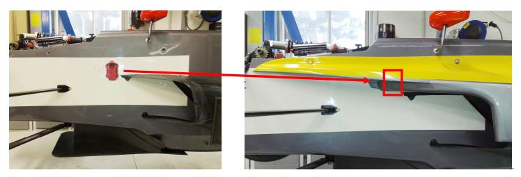
The transponder must be maintained with Velcro on the chassis, in front of the upper face of the left-hand radiator duct, inside the left-hand sidepod.
