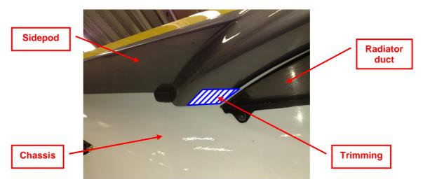
For this trimming, don't forget that usually when you remove the sidepod, you slide it forward before to remove it.
