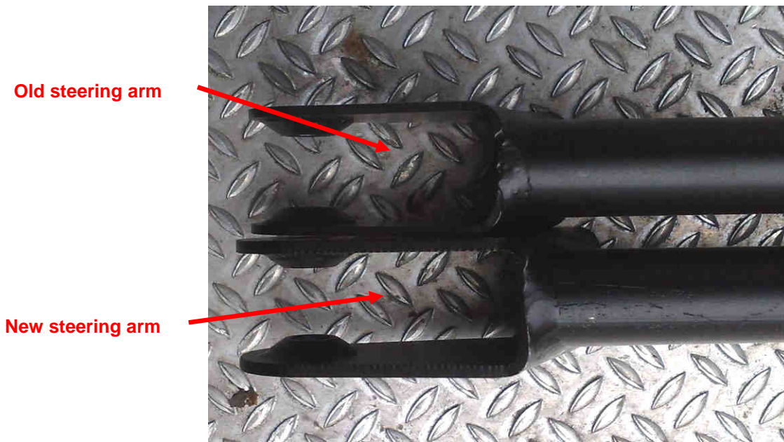
The clevis is thicker and wider
