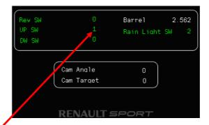
The switch must be activated (1 on the dashboard) after <u>a half stroke</u> of the shift paddle.
