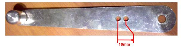
A new 6mm hole must be drilled 10mm below the original hole used to mount the cable rod end in order to easily pull the lever if needed.
