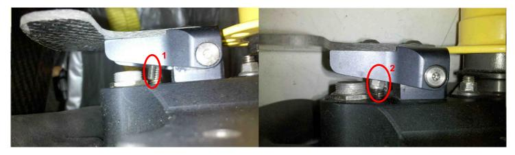
If you need to setup the stroke of the shift paddles, you must check directly on the dashboard when the steering wheel is connected:
