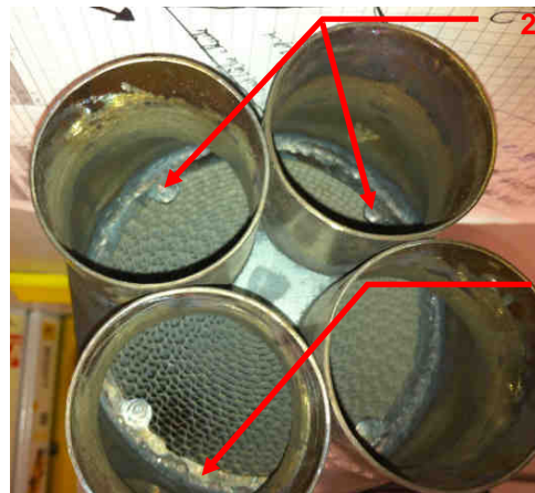
New design: 1 welded ring (1) + 4 welded pins added (2)
