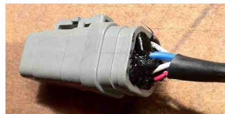
New connector body + wires twisted + silicone paste
