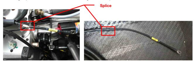
Moreover, Renault Sport strongly recommends you to modify the position of the GND Engine on the car, as shown below:
