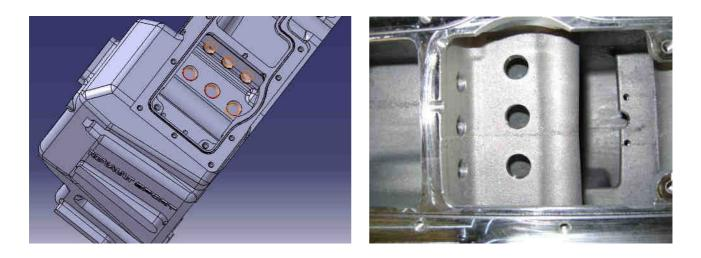
The oil tank must be completely disassembled and cleaned. Only the main housing must be sent to Sadev without any internal parts.
