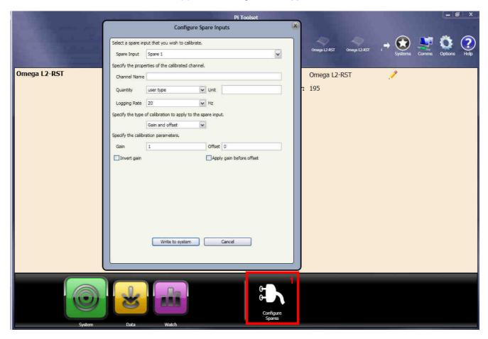
You must note that the spare channels can be calibrated by either entering a gain + an offset, or a table. It is also possible to set the channel name, the channel quantity & unit and the logging frequency.
