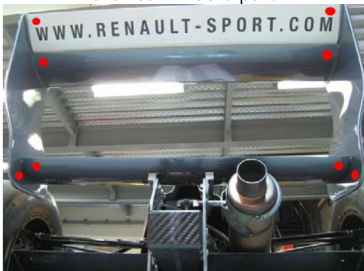
Rear wing: Lower part: two holograms underneath (left and right) Upper part: two holograms underneath (left and right) Upper flap: two holograms underneath (left and right) Endplate: one hologram inside, near the rear bottom
