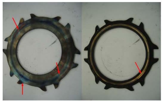
These colors on the pressure plates are an indication for extreme temperature build up in the clutch.
