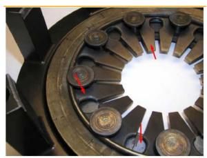
Defective cover through absorption of high temperature (the color of the spring is in range of purple to light blue = the high temperature is coming from the discs absorbed by the pressure plate than into the spring)
