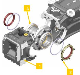
3.4.2. Disassembly/assembly of the components of the differential
