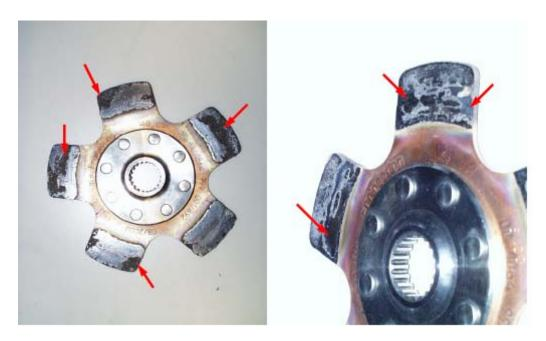
These are hot spots, where the material is losing adhesion to the support plate as a result of too much heat.
