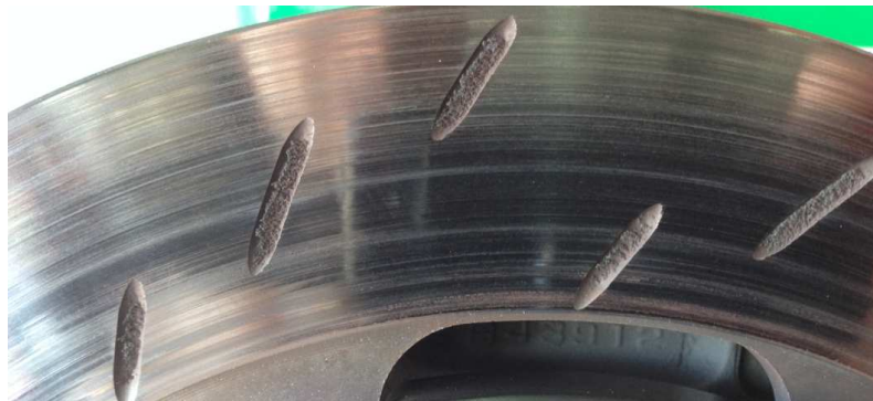
PFC 13 pad deposits clogging disc grooves
