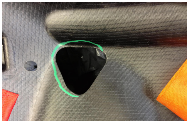
The green line represents the trimming required
